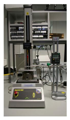
Fig. 2 Shows a digital force metre for measuring the strength of the adhesion
