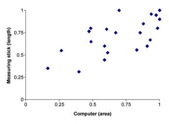
Fig. 4 Shows the correlation for adhesion coverage as assessed by a measuring stick versus digital computer analysis
