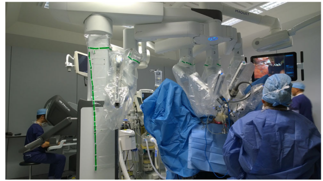
Fig. 3 The Da Vinci Xi surgical robot is sidedocked between the legs of the patient
