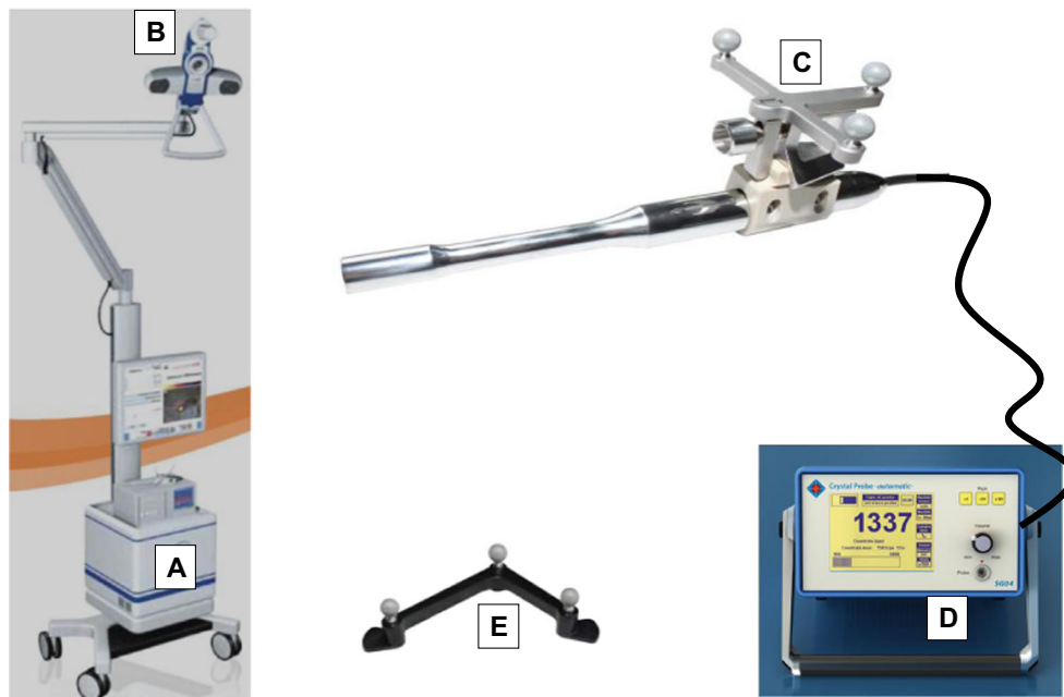
Fig. 1 The used freehand SPECT system used for laparoscopic sentinel lymph node detection. The system consists of an optical tracking system including the data-processing unit (part A), attached to an optical camera (part B) that is placed above the patient (similar to an operating light), and a hand-held gamma probe (part C) with little spheres serving as an optical reference (part E). The gamma probe is connected to a standard gamma detector (part D) used for sentinel lymph node biopsy. An optical patient
