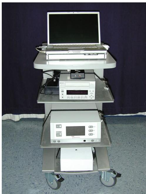
**Fig. 1** The VizAblate System. The ultrasound display is provided by the laptop, while the RF generator resides on the second shelf from the bottom
